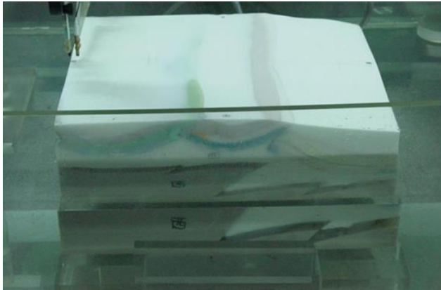
A shale reservoir model in a water tank to simulate seismic response
